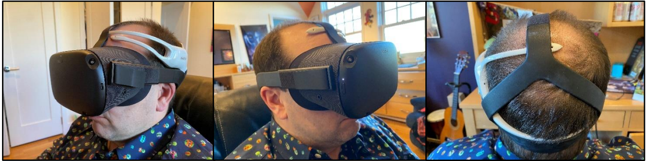
Figure 16: Testing apparatus combining the Emotiv Insight and the Oculus Quest
